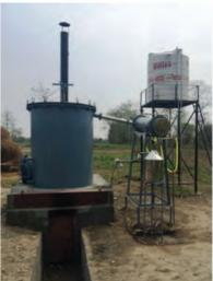
Mobile SS distillation units installed at ICAR Research Complex for NEH region
