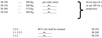
Seven days & 28 days cube test strength shall be given as per ISI for grade concrete even if mix is given by proportion.
